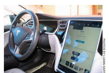
The inside of Brian Kopp's car shows the 17-inch touchscreen. Notice there is no ignition switch. The car starts when Kopp taps the brake.
