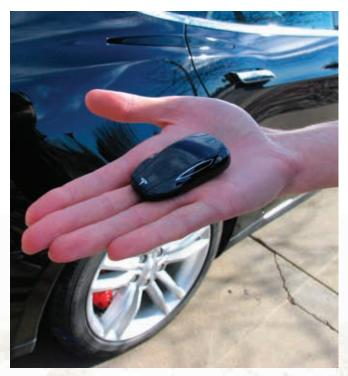
Brian Kopp shows the Tesla's key fob, which is shaped like the car. Tap on the trunk of the key fob and the trunk of the Tesla opens.
