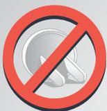
A study by Temple University found that **100%** of all 2-4 year olds were able to remove one type of plastic outlet cap **within 10 seconds**. Properly childproof your outlets by installing **Tamper-Resistant Receptacles**.
